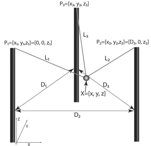
Fig. 2. Schematic of a three-cabled NIMS3D deployment showing the reference frame, end-effector location  $\vec{X} = [x, y, z]^T$ , the cable origins,  $P_i$ , the horizontal distances  $D_i$ , and cable lengths  $L_i$ ,  $i = 1, 2, 3$ .
