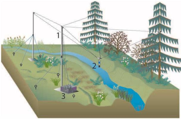
Fig. 1. Schematic of a four-cabled NIMS3D deployment showing: 1) infrastructure, consisting of poles and pulleys; 2) a generic sensor package; and 3) the motor control box.
