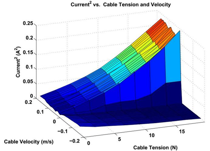
Fig. 11. Square of motor current shown as a function of cable velocity and torque. Positive cable velocities indicate raising a load, while negative velocities indicate lowering a load.
