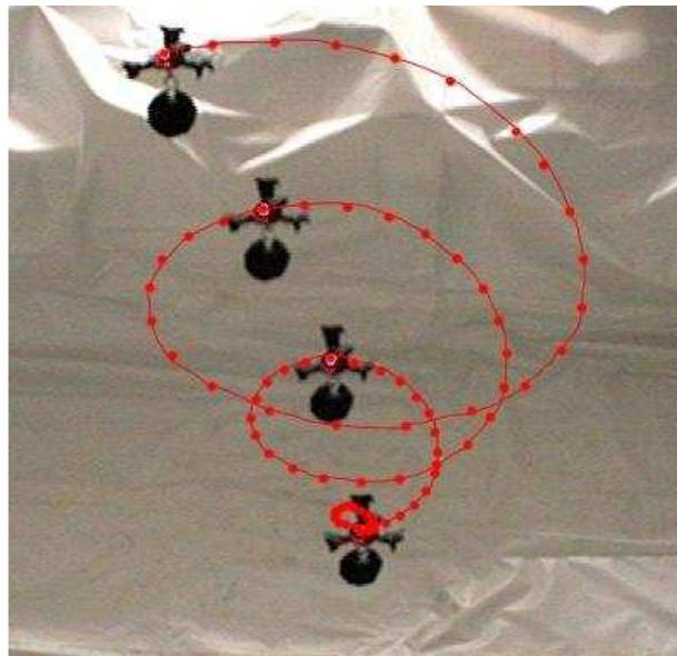
Fig. 9. Time-lapse image of NIMS3D executing a spiral trajectory. Dots show node position at evenly spaced time intervals. In addition, the node is pictured four times along the trajectory.
