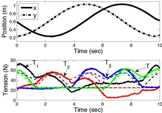
Fig. 5. Experimental tension distribution results showing cable tensions and end-effector position during execution of a circular trajectory. Commanded tensions are shown as dashed lines.
