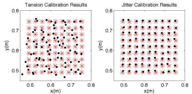
Fig. 6. Calibration results for (left) tension-based and (right) jitter-based calibration methods. Stars indicate actual position, while dots show calibration results.
