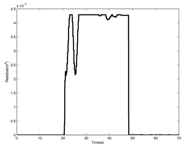
Fig. 9. Trace of drift-detection residual during the drift-correction experiment.
