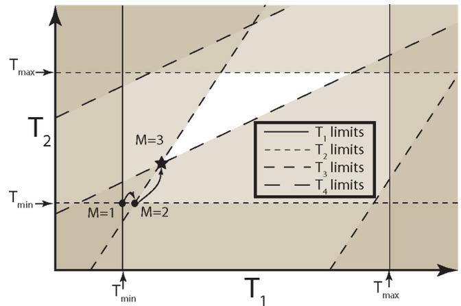
Fig. 4. Example of the iterative tension solver. For iteration number  $M = 1$ ,  $\mathbf{f}_1 = [T_{\min} \ T_{\min}]^T$ , but two constraints are violated. The next point is found by moving along the  $T_2 = T_{\min}$  edge toward the first violated constraint. After this iteration, only one violated constraint remains, and we move along the  $T_3$  constraint to the optimal operating point  $\mathbf{f}_1^*$ .
