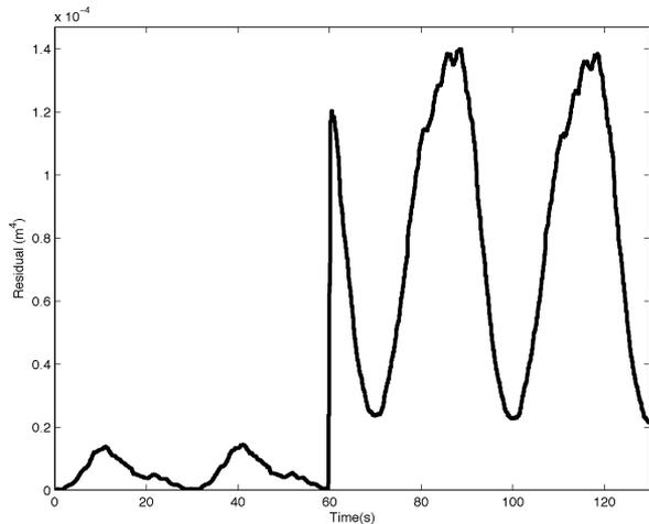
Fig. 7. Trace of the residual from the drift-detection algorithm during execution of a circular trajectory. At  $t = 59.5$  s, a drift of 2.44 cm is introduced in the length of cable 4.
