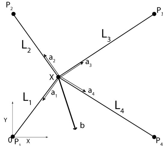
Fig. 3. Schematic of a NIMS-PL configuration showing unit vectors  $a_i$ , cable origins  $P_i$ , end-effector position  $\mathbf{x} = [x \ y]^T$ , and an example desired force vector  $\mathbf{b}$ .
