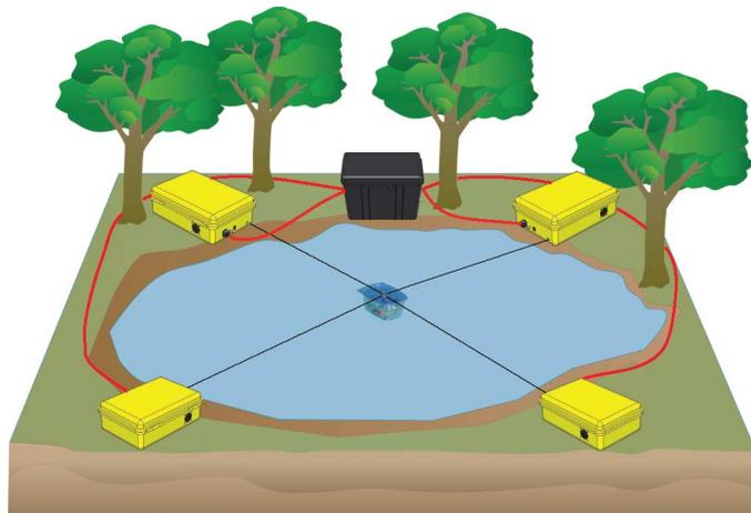
Fig. 1. Schematic of a NIMS-PL deployment showing four actuator units, the motor control box, and a buoyant end-effector.
