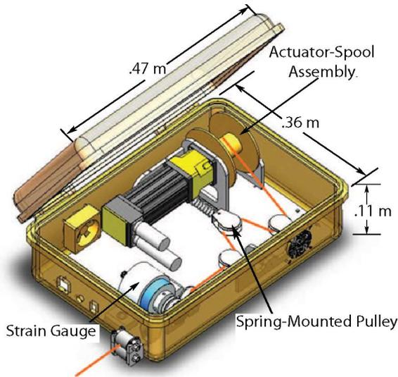
Fig. 2. Actuation module showing the actuator-spool assembly, tension gauge, and spring mounted pulley.
