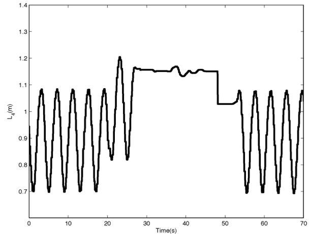
Fig. 8. Trace of  $L_4$  showing a large offset caused by cable drift and subsequent drift correction via jitter-based self-calibration.
