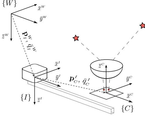
Fig. 1. Relationship between the world  $\{W\}$ , IMU  $\{I\}$ , and omnidirectional camera  $\{C\}$  reference frames. The goal of the calibration procedure is to determine the transform  $(\mathbf{p}_C^I, \bar{q}_C^I)$  between the camera and IMU, using accelerometer and gyroscope data and camera images of static point landmarks (red stars) in the immediate environment.
