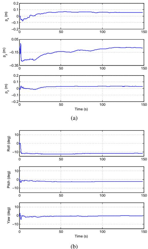
Fig. 4. (a) Evolution of the IMU-to-camera translation estimate over the calibration time interval (along the  $x$ ,  $y$  and  $z$  axes of the IMU frame, from top to bottom) for the self-calibration procedure. (b) Evolution of the IMU-to-camera orientation estimate (for the roll, pitch and yaw angles that define the orientation of the camera frame relative to the IMU frame, from top to bottom) for the self-calibration procedure.
