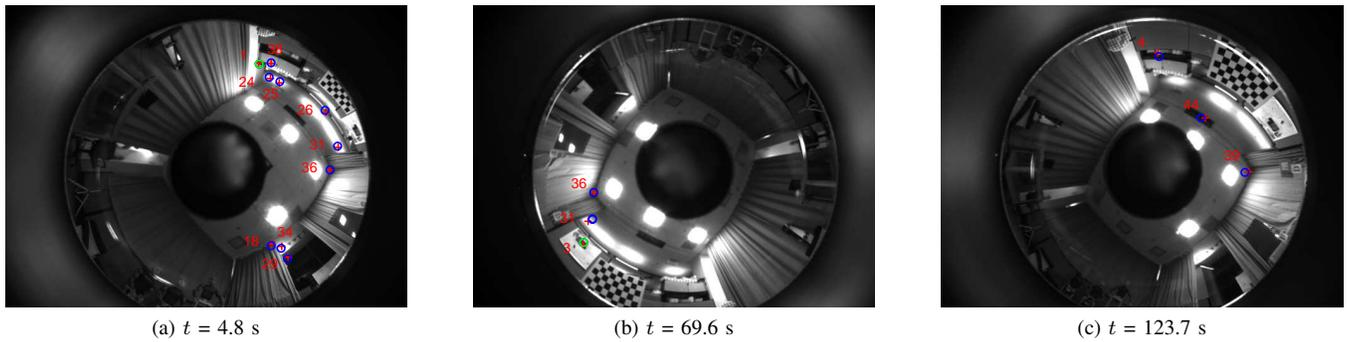
Fig. 3. Images from the self-calibration data set, at times  $t = 4.8$  s,  $t = 69.6$  s and  $t = 123.7$  s from left to right, respectively. The measured image locations of the identified landmarks are shown as red crosses, and the predicted locations are shown as blue circles. Green circles identify anchor landmarks, which we used to fix the orientation of the world frame. The planar calibration target was used only to determine the initial and final positions of the camera.
