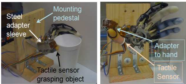
Figure 5: Hand/Sensor assembly: the thumb of the hand is removed and a shore A 60 rubber socket is placed over the stump and hard-bolted to the sensor via a steel adapter
