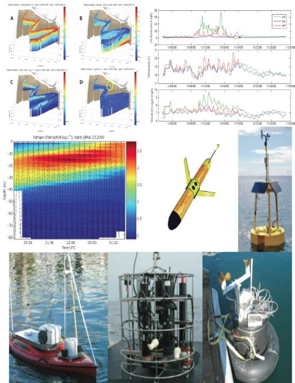
**Figure 1** Data and sensors of the embedded coastal sensor network. Components include (bottom row from the left) an autonomous surface vessel, traditional sampling platforms (Niskin bottle rosette and sensors), custom buoys for quiescent environments, a Webb Slocum glider (center photo) and ocean moorings (middle right). Data outputs include 2-D and 3-D spatial reconstructions (middle and upper left, resp.) and temporal patterns (upper right) of physical, chemical and biological features.
