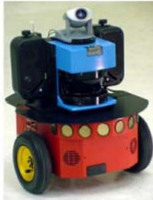
**Figure 1:** The Pioneer mobile robot base used in the experiments. Shown is the laser (the blue box), camera (mounted on top of the laser), and speakers (mounted on each side of the laser).
