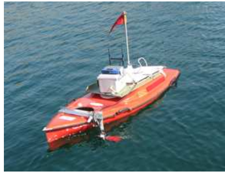
Fig. 2. The USC RESL Autonomous Surface Vehicle used for the experiments reported here.
