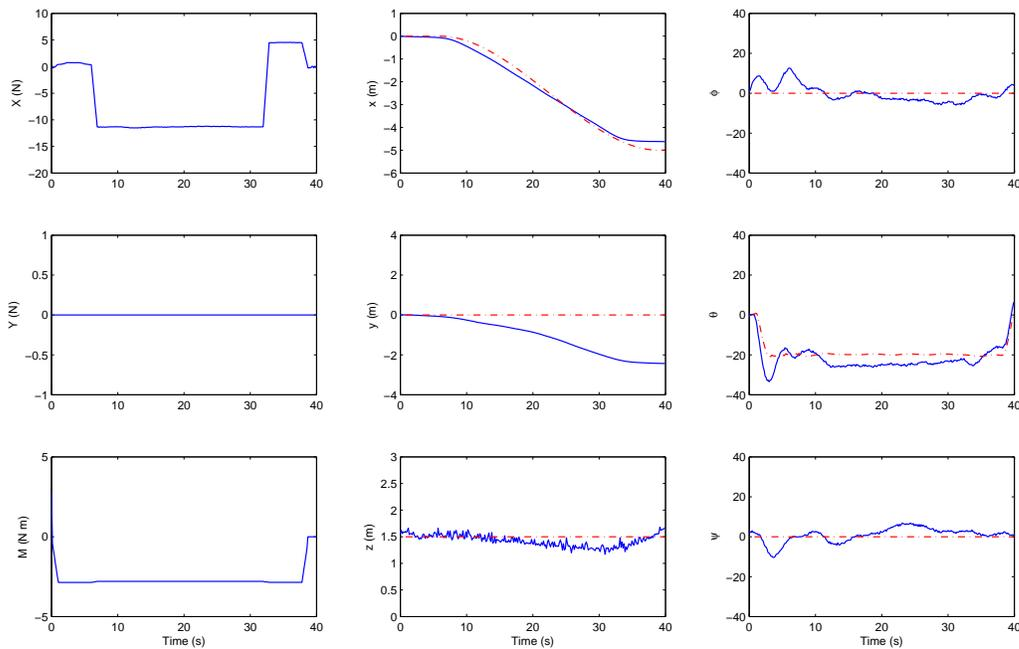
Fig. 10. Strategy Two: Horizontal survey. Solid (blue) line represents actual evolution, dash-dot (red) line represents the theoretical evolution.
