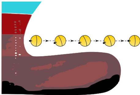
Fig. 7. Side view of a bulbous bow on a ship. Also depicted is the linear trajectory for the inspection of the top of a bulbous bow.
