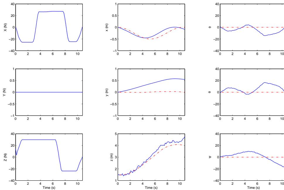
Fig. 9. Strategy One: Semi-circle trajectory. Solid (blue) line represents actual evolution, dash-dot (red) line represents the theoretical evolution.
