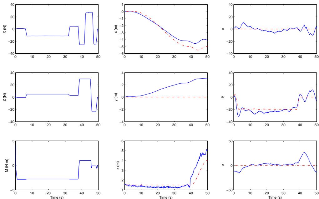
Fig. 11. Strategy Three: Concatenation of the semi-circle trajectory and the horizontal survey. Solid (blue) line represents actual evolution, dash-dot (red) line represents the theoretical evolution.
