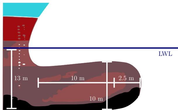
Fig. 4. Side view of a bulbous bow on a ship and its dimension.
