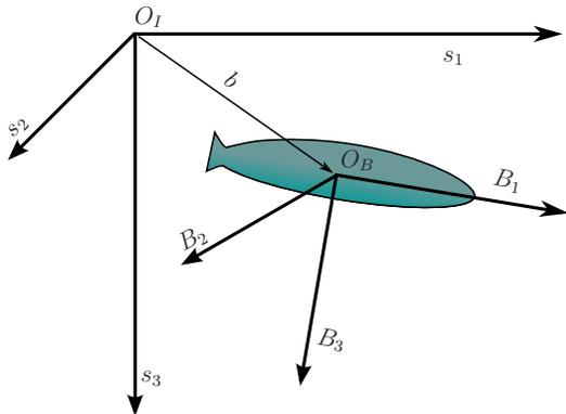
Fig. 2. Earth-fixed and body-fixed coordinate reference frames.
