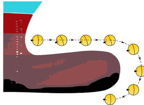
Fig. 8. Overall path for complete inspection of a bulbous bow.
