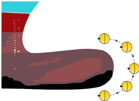
Fig. 5. Side view of a bulbous bow on a ship. Also depicted is the semi-circle trajectory for the inspection of the front of a bulbous bow.
