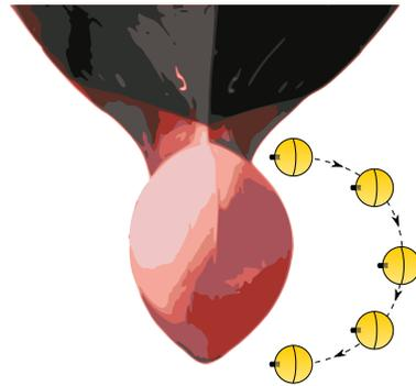
Fig. 6. Front view of a bulbous bow. Also depicted is the trajectory to survey the sides of the bulb.
