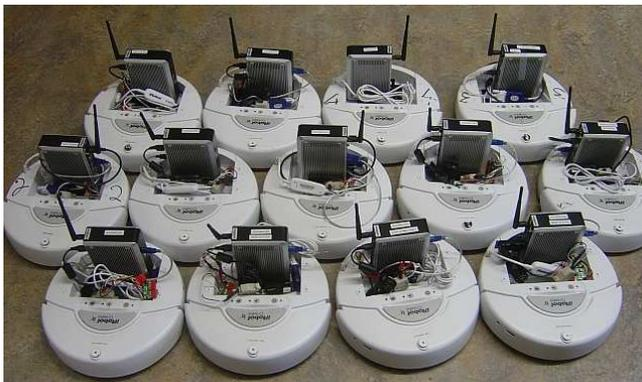
**Fig. 2** Team of Creates which depicts our robot platform - the iRobot Create with an Ebox
