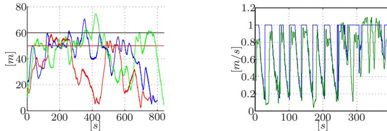
**Fig. 5** a) Plot of the relative distance between the vessels during three field trials. The leader-follower strategy is activated when the distance is greater than 50  $m$ . The leader has to stop and wait for the follower when their distance is greater than 60  $m$ ; b) Plot of one of the vessels' desired and measured velocity during the first 400 s of an experiment.
