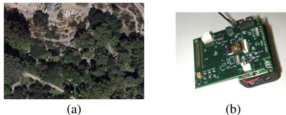
Figure 1. (a) An aerial view of the garden (b) Cyclops camera with an attached Mica2 Mote
