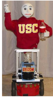
Fig. 1: Robot test-bed: Human-like torso mounted on the mobile base
