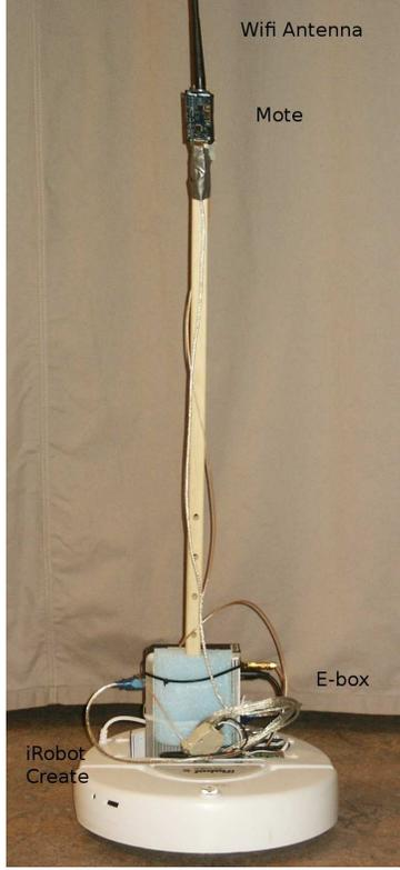
Fig. 8: Create fitted with raised antenna
