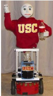
Figure 1. Human-like torso mounted on a mobile base
