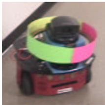
Figure 1: Pioneer Robot with Color Markings
