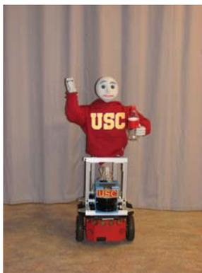
Figure 1: Humanoid torso mounted on a mobile base (Bandit II - the hands-off therapist robot designed at the USC Interaction Lab)
