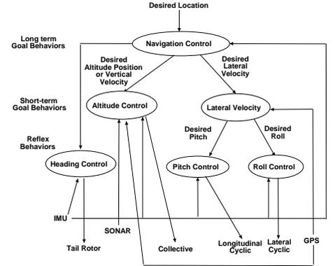
**Fig. 2.** Behavior-Based Controller
