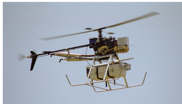
Fig. 1. The AVATAR, USC's robotic helicopter.
