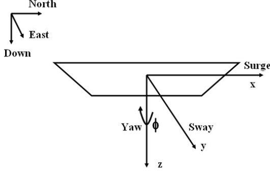
Fig. 4. Coordinate System used in Marine Navigation
