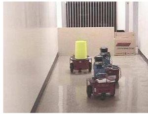
(b) 2 robots tracking 1 target
