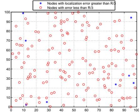
Fig. 2. Edge Effects: For a specific instance (with Num nodes = 150 and Radius of communication = 20) the empty circles denote nodes localized within  $(R/3)$  distance from actual location and the stars denote nodes localized with error greater than  $(R/3)$
