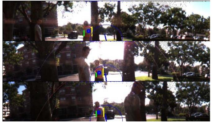
Fig. 6. Output from the omnica during tracking among trees: the robot is following the person in the middle (top frame - small circle indicates target position estimate), while another person (from the left) is crossing the path between the robot and the first person
