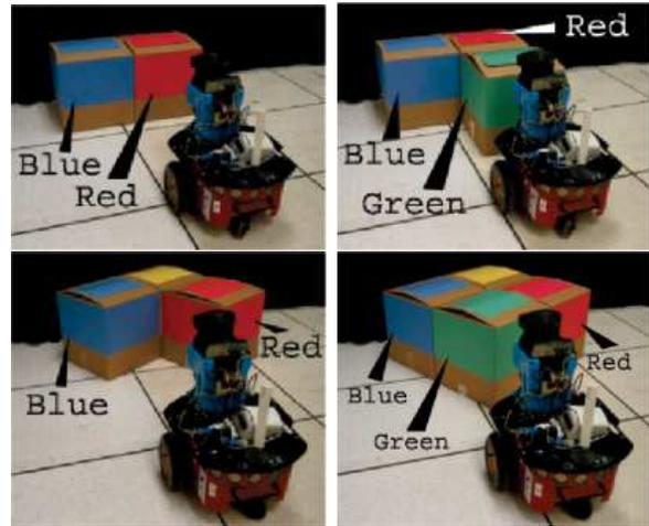
Fig. 4. Example observations and actions in the construction domain. (top left) Robot in position to make observation  $\langle \text{FLUSH R B} \rangle$ . (top right) Immediately after robot performs action  $\langle \text{G RIGHT FLUSH R B} \rangle$ . (bottom left) Robot in position to make observation  $\langle \text{CORNER R B} \rangle$ . (bottom right) Immediately after robot performs action  $\langle \text{G CORNER R B} \rangle$ .
