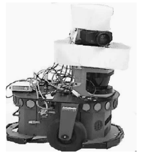
Fig. 4. A robot with laser and panned camera, the lens peering out through the hole in the color helmet.
