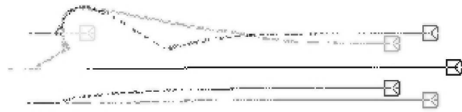
Fig. 7. A trial of 6 robots in a circle (hexagon); one is terminated, and the rest adapt to a 5-circle (pentagon).
