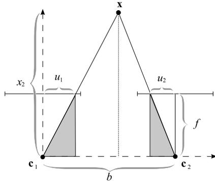
Figure 2: Standard model of linear perspective projection for stereo triangulation with axis aligned cameras.
