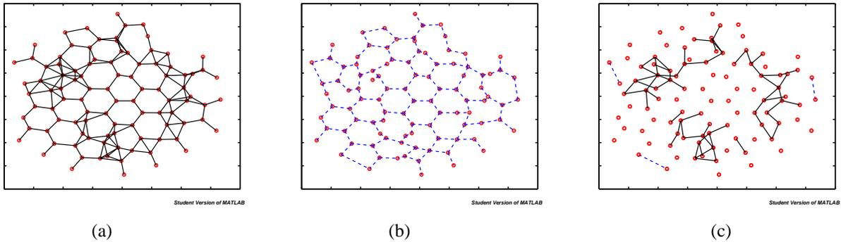
**Fig. 11.** Comparison of communication graph and corresponding RNG [**Incremental Deployment, 100 nodes,  $\theta = \frac{2\pi}{3}$ , large error**] a) communication graph b) RNG c) Dashed lines indicate edges in RNG that are not in communication graph. Dark lines indicate edges in communication graph that are not in RNG.
