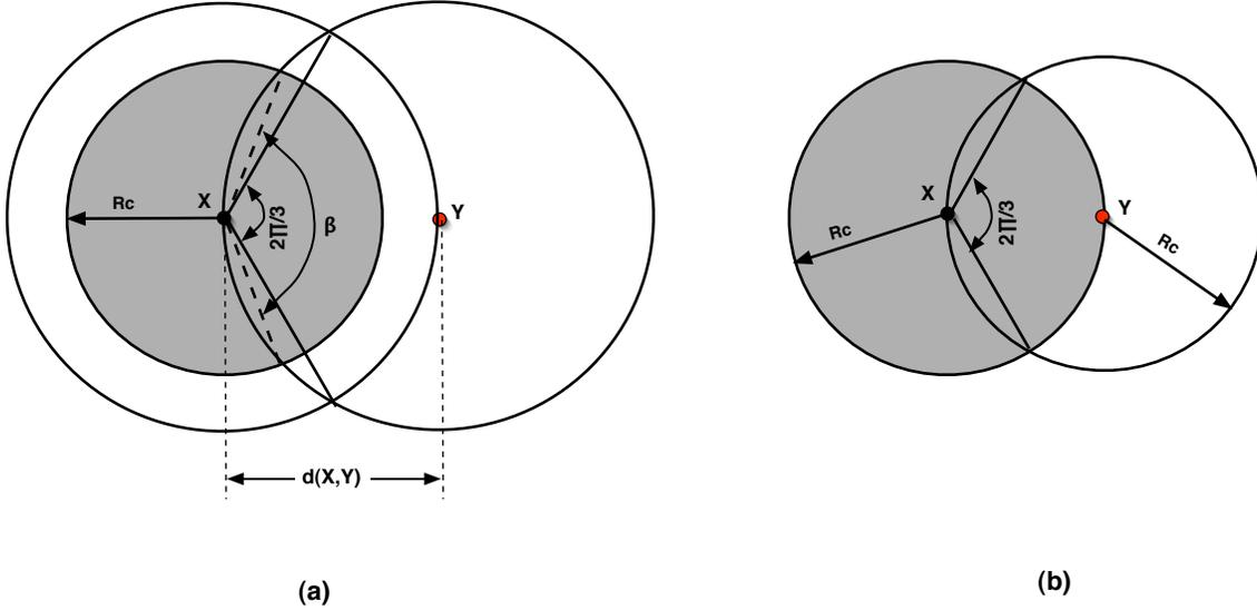
**Fig. 2.** RNG sector condition. a) The circle of radius  $d(X, Y) > R_c$  subtends an angle of  $\frac{2\pi}{3}$  at  $X$ . The lune contains an area larger than a  $\frac{2\pi}{3}$  sector. b) The limiting case, when  $d(X, Y) = R_c$ .
