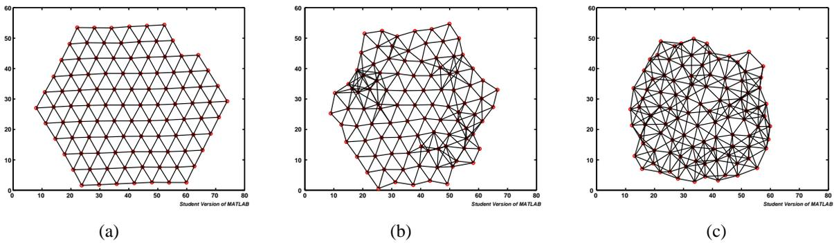
**Fig. 7.** Topologies obtained for  $\theta = \frac{\pi}{3}$  with 100 nodes and  $R_s = R_c = 8m$  using a) Incremental deployment with small error b) Incremental deployment with large error and c) Distributed deployment
