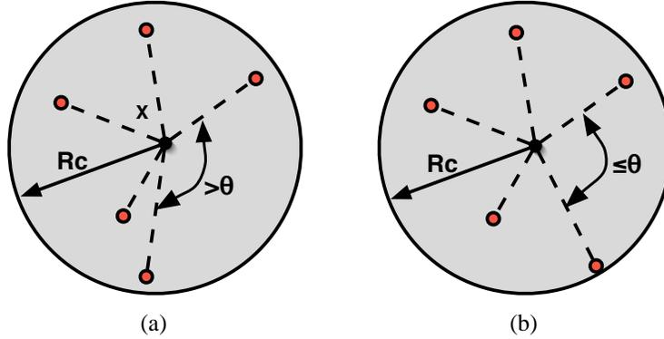
**Fig. 1.** Illustration of the NET condition. In a), node X has one sector greater than a given angle  $\theta$  with no neighbor. It does not satisfy the NET condition. In b), the largest sector with no neighbors is smaller than  $\theta$ , satisfying the NET condition
