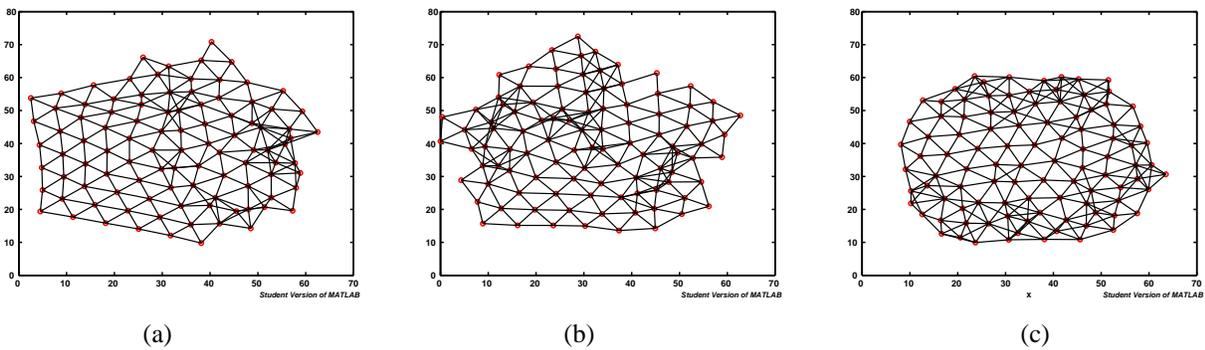
**Fig. 8.** Topologies obtained for  $\theta = \frac{2\pi}{5}$  with 100 nodes and  $R_s = R_c = 8m$  using a) Incremental deployment with small error b) Incremental deployment with more error and c) Distributed deployment
