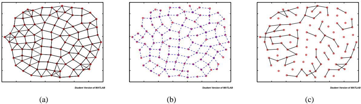
**Fig. 12.** Comparison of communication graph and corresponding RNG [**Distributed Deployment, 100 nodes,  $\theta = \frac{2\pi}{3}$** ] a) communication graph b) RNG c) Dashed lines indicate edges in RNG that are not in communication graph. Dark lines indicate edges in communication graph that are not in RNG.
