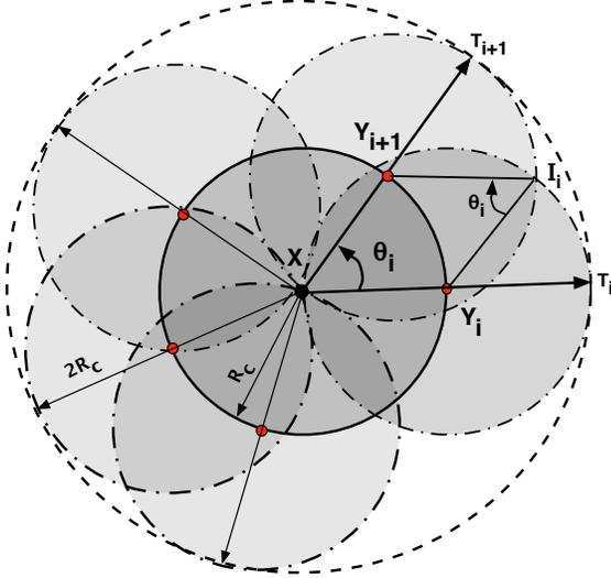
**Fig. 6.** Coverage with  $k$  nodes placed on the communication perimeter of node  $X$ . The shaded area is the total coverage.
