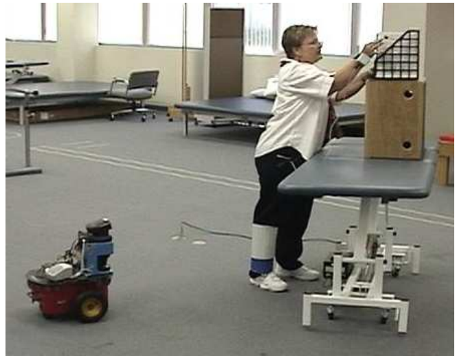
Fig. 2. The robot and a stroke patient during an experiment, where the desired activity is to shelve books. The arm sensor is visible on the patient’s right forearm; the patient also wears laser fiducials on her leg to make it easier for the robot to recognize and follow her.
