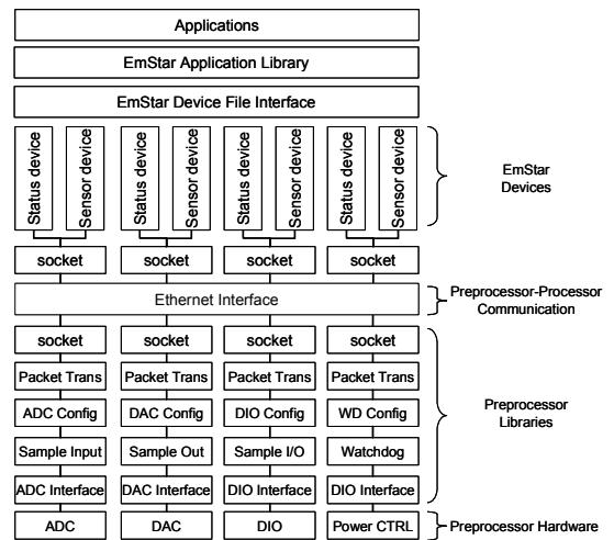
**Figure 4.** The NIMS Processor-Preprocessor software architecture is shown. This architecture exposes the standard EmStar status and sensor device file interfaces to each of the analog input (ADC), analog output (DAC), and digital input/output (DIO) to applications. An additional interface may be added as well for watchdog fault recovery functionality.
