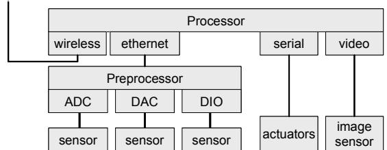
**Figure 3. The NIMS Processor/Preprocessor architecture showing sensor interfaces supported by the preprocessor and actuator and image sensor interfaces supported by the processor.**
