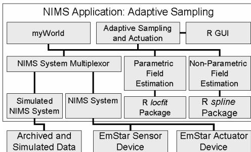
**Figure 6.** The architecture for the embedded R statistical computing environment on the NIMS node is shown. NIMS R code applications may access sensors and actuators in real-time field, simulated, or archived data creating the myWorld application environment.
