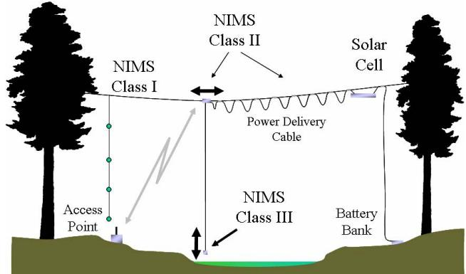
**Figure 1.** NIMS Class I, II, and III architectures are shown in schematic view, deployed in a forest environment for microclimate and water system monitoring. NIMS Class II devices move horizontally and control elevation of attached NIMS Class III nodes. Class I nodes suspended from the infrastructure are shown as well.
