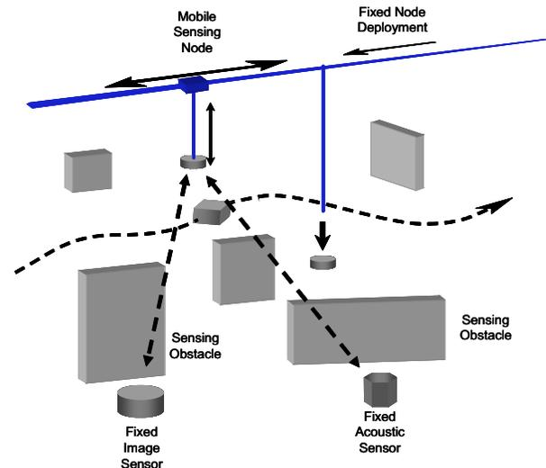
**Figure 2.** NIMS infrastructure permits mobile sensor nodes to precisely reconfigure to both probe and then reduce sensing uncertainty. NIMS distributed operations engage both mobile and fixed embedded sensor nodes.
