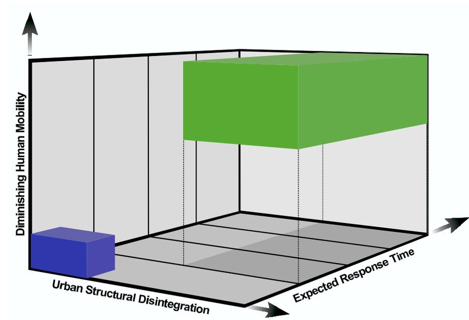
Figure 1: A decomposition of the task space for disaster recovery robotics. The small and large blocks represent evacuation assistance and USAR tasks, respectively. The space spanned by the axes indicates conditions of the survivors; some regions are infeasible, and no survivors are assumed to exist outside the axes.
