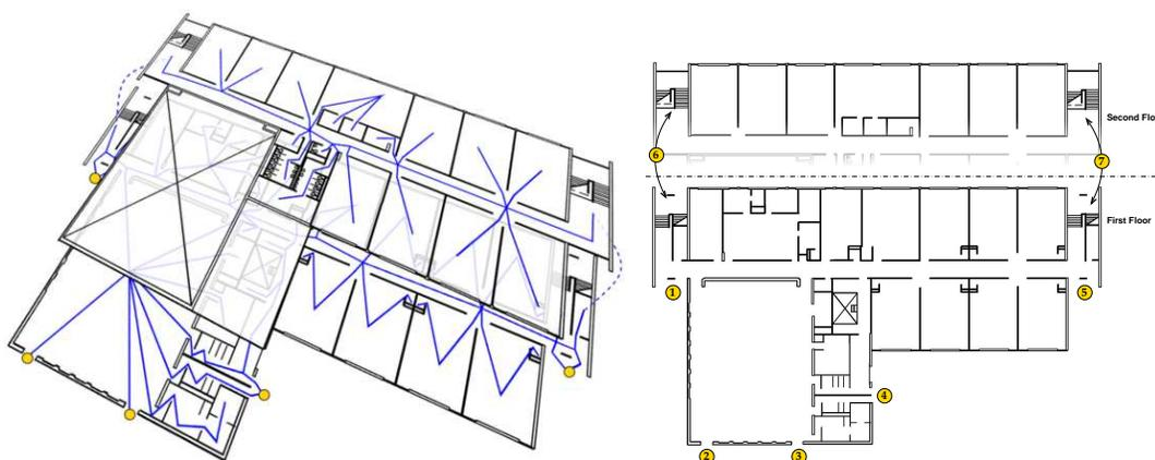
Figure 4: A representation of one of the multi-floored test environments used for beacon deployment. The dots mark pieces of information added by the operator, in this case emergency exits and stairwell links. The image on the left includes a topological overlay for the environment. On the right, the emergency exits are numbered 1-5 and the connection stairways 6 and 7 (the second floor is only partially shown).
