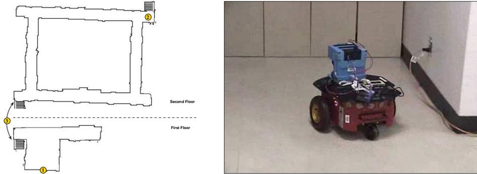
Figure 5: The map used with physical robots. Exits marked 1, 2. The connection labeled 3 is a stairwell. The ActivMedia Pioneer DX2 is shown moving toward the top of the stairwell.
