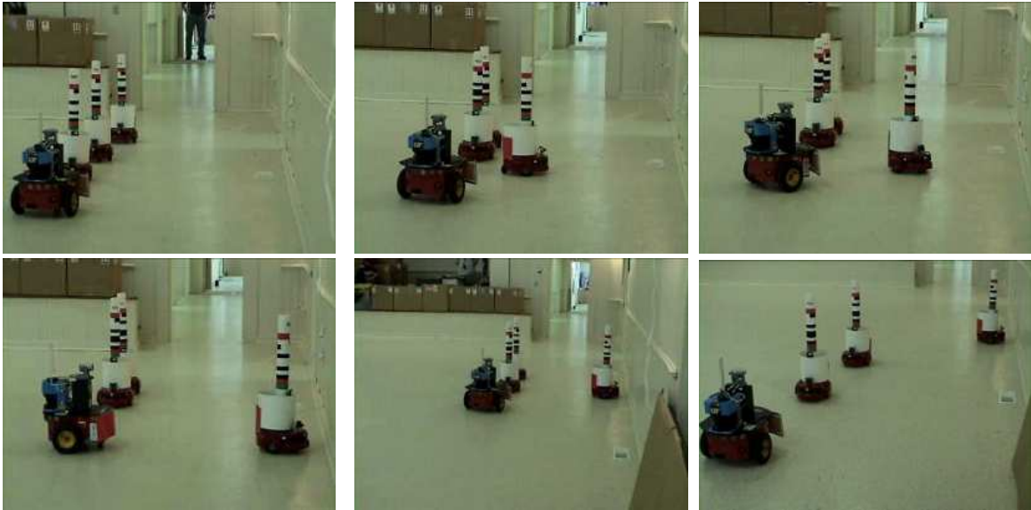
Figure 8: Deployment of a sensor robot using assistive navigation: the lead robot first guides and then directs the sensor robot into position.
