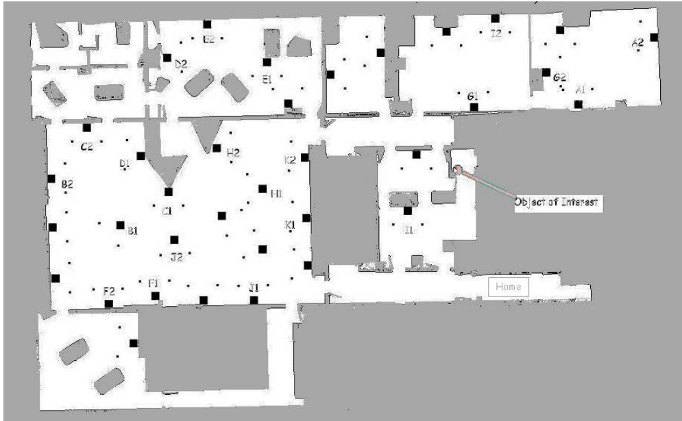
Figure 9: Autonomously planned sensor net positions (black squares) and planned leader way-points associated with each sensor position (small dots).
