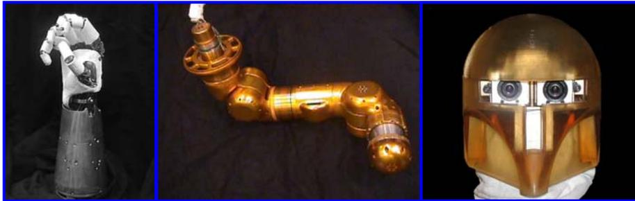
Fig. 3. The Robonaut hand, arm, and head
