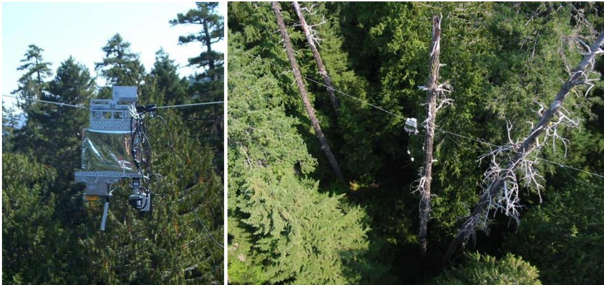
Figure 7. (Left Panel) A Class II NIMS Node system deployed in a forest environment. This node includes embedded computing, wireless networking, horizontal transport, image sensing. This node also supports a vertically suspended meteorological sensing Class III Node carrying atmospheric temperature, relative humidity, and photosynthetically active radiation (PAR) sensor devices. Wireless links provide access between the nodes and conventional wide area networks.
