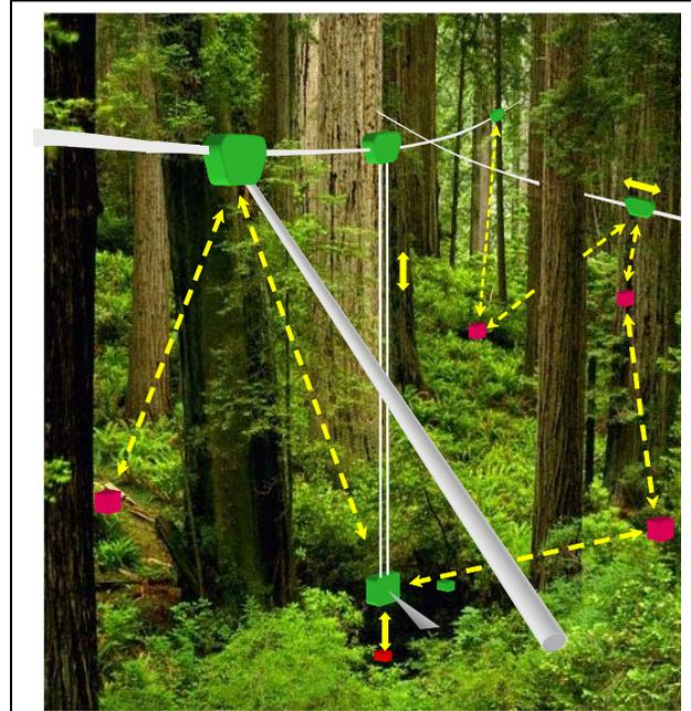
Figure 1. Networked Infomechanical Systems (NIMS) introduces a hierarchy of fixed and mobile sensing nodes and infrastructure enabling access to complex, three dimensional environments. NIMS mobility provides novel methods for establishing self-awareness of sensing uncertainty. Further, examples of new NIMS distributed services include node transport, physical sample acquisition, energy harvesting and delivery, wireless network relay functions, and many others.
