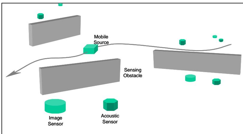
Figure 2. Environments inherently present obstacles to sensing, as shown here for distributed imaging and acoustic sensors. Unpredictable source motion leads to obscuration of the source from sensors.
