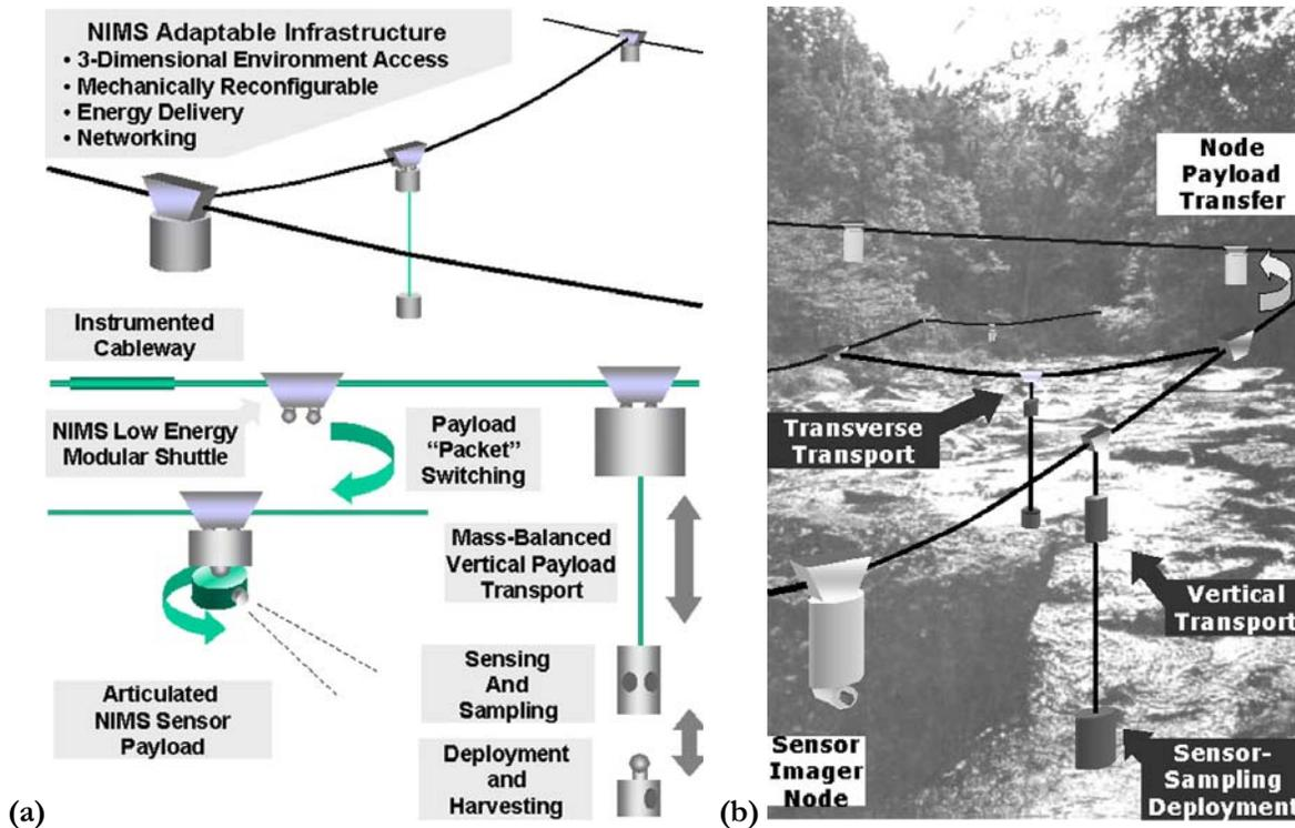
Figure 3. (a) NIMS Systems include fixed and mobile nodes along with instrumented and adaptable infrastructure. NIMS nodes may be fixed to the infrastructure, may move on the infrastructure, or be delivered to locations and recovered by other nodes. (b) A schematic view of a NIMS deployment in a riparian stream environment with distributed sensing, sampling, and node transport
