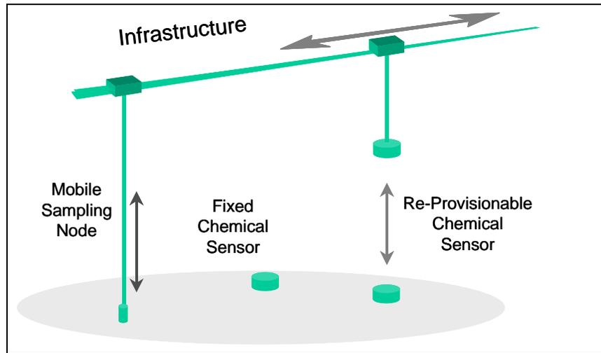
Figure 5. In addition to physical sensing, NIMS enables physical sampling where mobile devices may acquire samples according to an event-driven or scheduled algorithm and convey samples to centralized sample analysis facilities (that may include remote laboratory analysis). NIMS also permits re-provisioning of in situ sensors that may be otherwise limited by a short operating lifetime in the medium.
