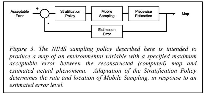
Figure 3. The NIMS sampling policy described here is intended to produce a map of an environmental variable with a specified maximum acceptable error between the reconstructed (computed) map and estimated actual phenomena. Adaptation of the Stratification Policy determines the rate and location of Mobile Sampling, in response to an estimated error level.
