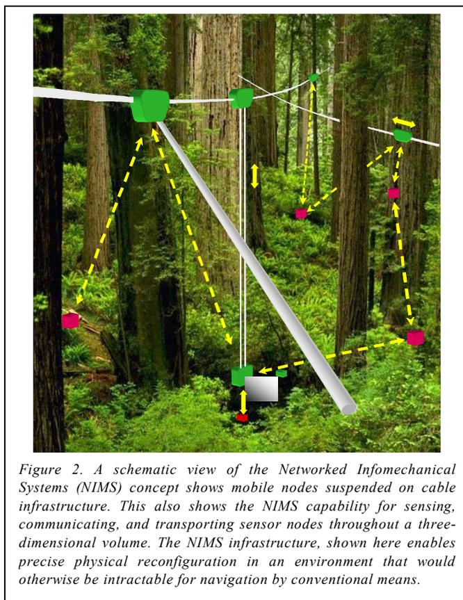
Figure 2. A schematic view of the *Networked Infomechanical Systems (NIMS)* concept shows mobile nodes suspended on cable infrastructure. This also shows the NIMS capability for sensing, communicating, and transporting sensor nodes throughout a three-dimensional volume. The NIMS infrastructure, shown here enables precise physical reconfiguration in an environment that would otherwise be intractable for navigation by conventional means.
