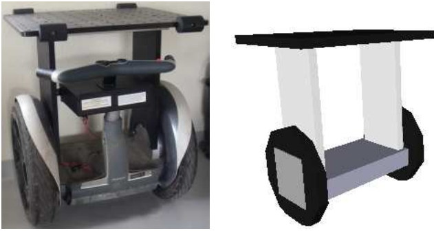
Fig. 4. Above is a real SegwayRMP and its model in Gazebo below.
