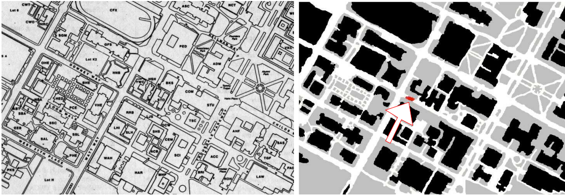
Fig. 5. (a) Scanned map of the USC University Park campus. (b) Induced map, showing free space (white), occupied space (black), and semi-occupied space (gray). The particle filter estimate is indicated by the arrow.
