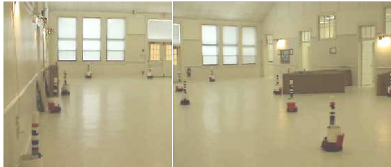
Fig. 7. Physical robots deployed according to the results of the autonomous planning process for the environment shown in Figure 6.
