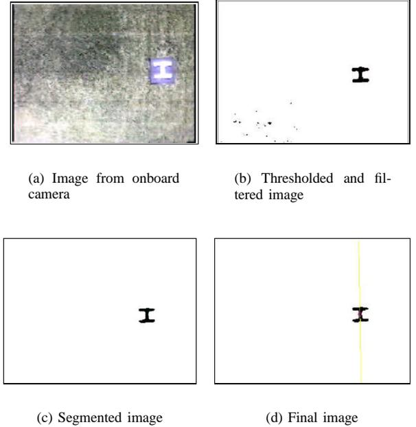
Fig. 3. Image processing results. Image (a) is captured in flight from the downward-pointing camera on the helicopter
