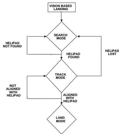
Fig. 2. The state transition diagram for landing.
