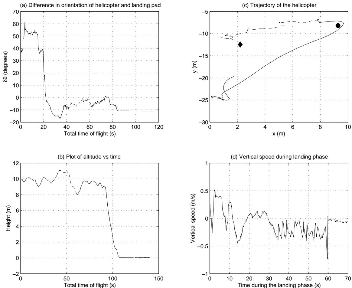
Fig. 6. Vision algorithm in conjunction with the landing controller when the helipad is moved.
