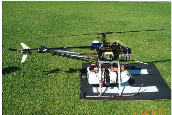
Fig. 1. The USC AVATAR (Autonomous Vehicle Aerial Tracking And Reconnaissance) after landing on a helipad
