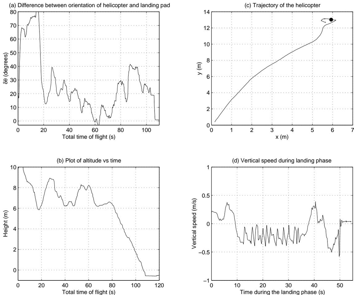
Fig. 5. Performance of the vision algorithm in conjunction with the landing controller for a stationary helipad.
