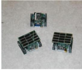
(a) robots with solar cells
