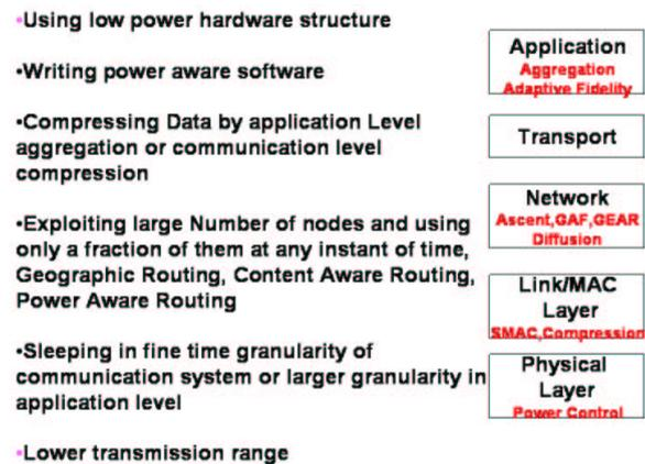
Figure 1: Low power network design techniques
