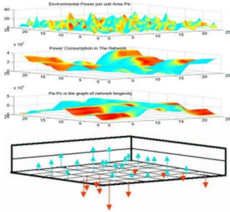
**Figure 2: The top figure is available environmental power, the next figure is power consumption. The difference of the two is an important factor in longevity of the network. The last figure shows discrete samples of power distribution across the network nodes.**
