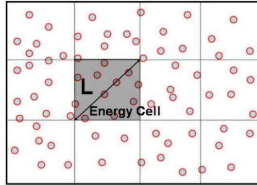
**Figure 3: Energy Cell defines the territory of each robot and its zone of service. The area spanned by the network is divided into Energy Cells. The number of robots per cell depends on the number of static client nodes, the rate of their energy consumption and available environmental energy**
