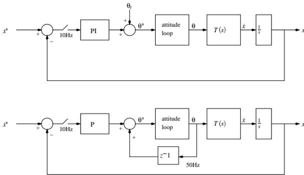
Figure 8: Different control structure of CSIRO(top) and USC(bottom) helicopters.
