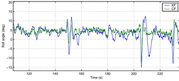
Figure 6: KF and CF comparison at estimating roll angle.
