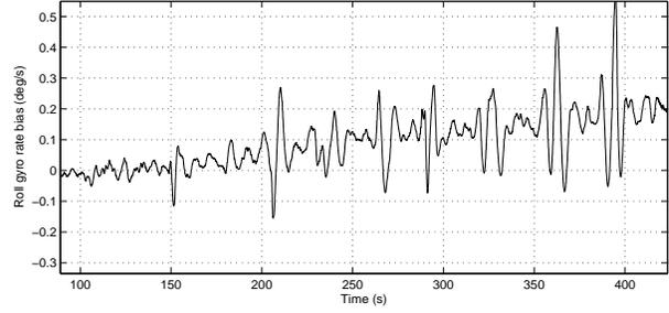
Figure 7: Roll gyro rate bias estimated by KF.
