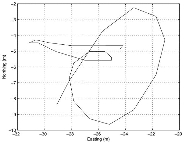
Figure 9: DGPS position during hover (velocity control only).
