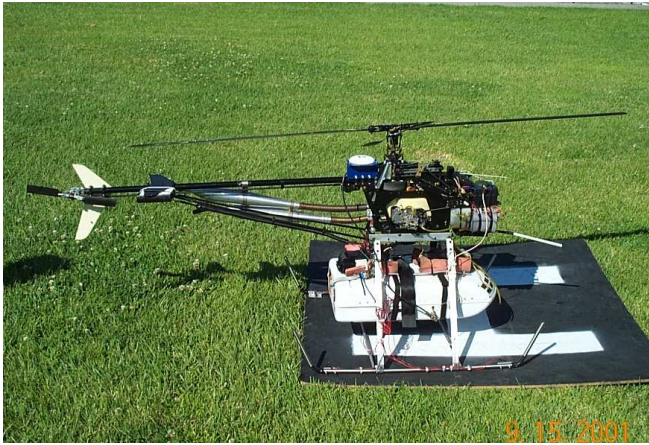
Figure 1: AVATAR (Autonomous Vehicle Aerial Tracking And Reconnaissance) after landing on a stationary helipad
