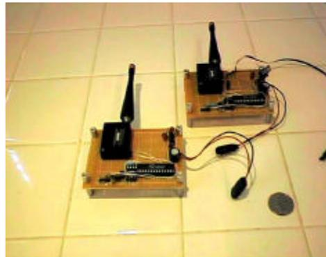
**Figure 2. A pair of communication modules**
