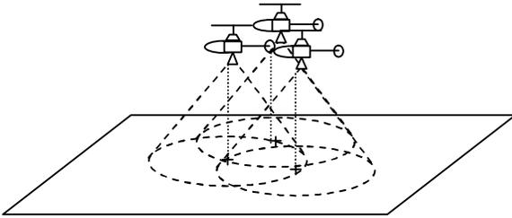
**Figure 5. Vision based relative localization**
