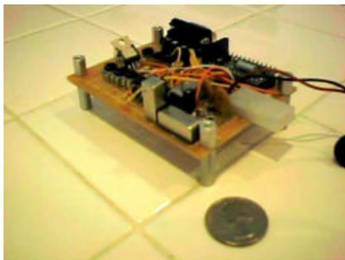
**Figure 4. Inertial Measurement Unit**
