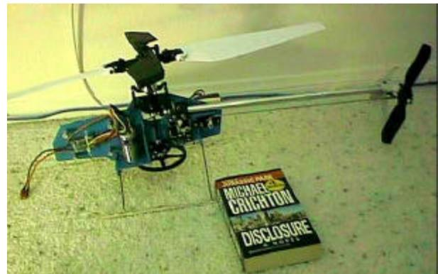
Figure 1. Electric LMH-110 Model Helicopter
