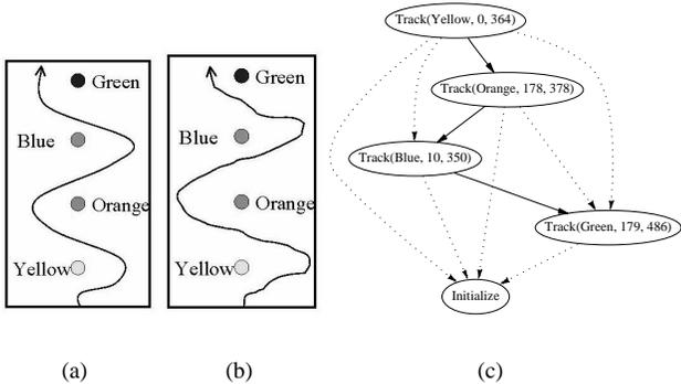
**Figure 7. The “Slalom” task: (a) Experimental setup; (b) Approximate robot trajectory; (c) Task representation learned from the demonstration of the Slalom task**
