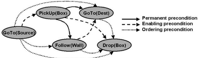
**Figure 2. Example of a behavior network**
