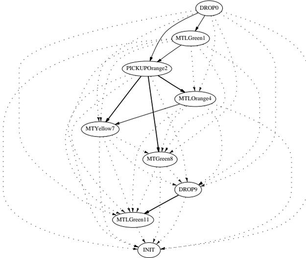
**Figure 11. Task representation learned from human demonstration for the “Object manipulation” task**
