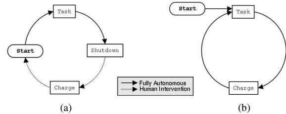
Figure 1. Robot task cycle comparison.
