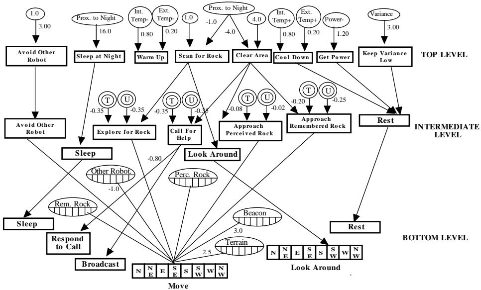
**Figure 2.** FFH system for BISMARC. All weights on the arcs are 1.0 unless otherwise indicated. Notation for symbols is that of Tyrrell.<sup>17</sup> See text for a detailed discussion.
