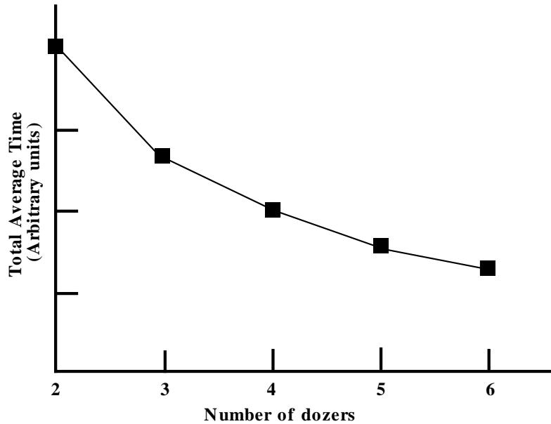
**Figure 3.** Average total mission time for 48 simulation trials versus the number of dozers in each trial. Time is in arbitrary simulation units with an average time of 3 weeks, 4 days for two dozers.
