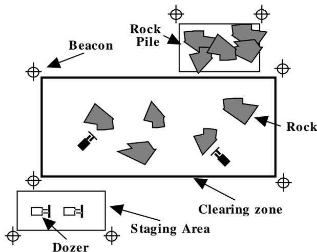
**Figure 1.** Beacons delimited site for autonomous clearing operation. Site size is 100 m×50 m.
