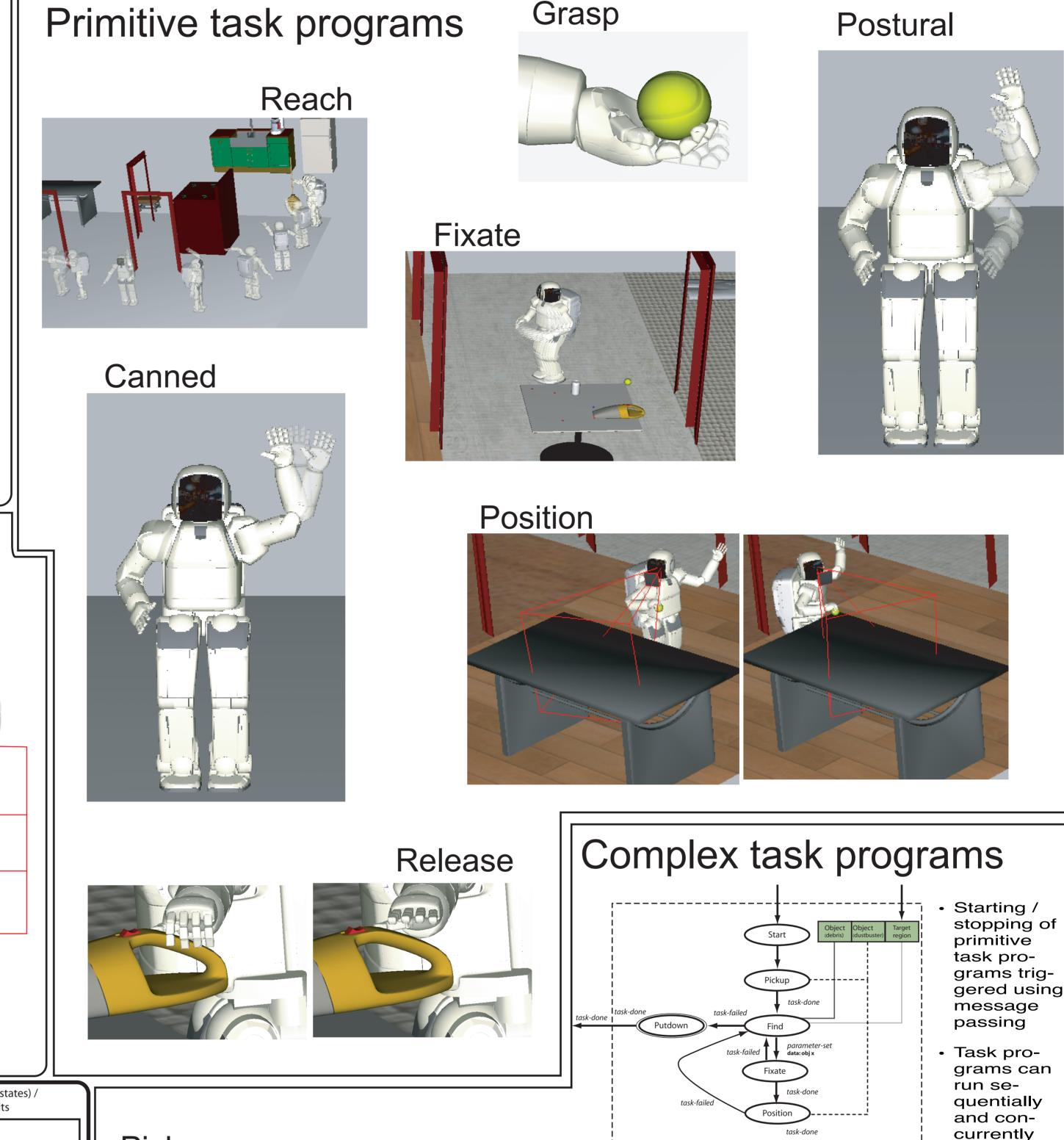
These programs can be manually combined to perform complex tasks or learning can be used to automatically determine how to sequence and combine them (e.g., [Bentivegna 2004])
