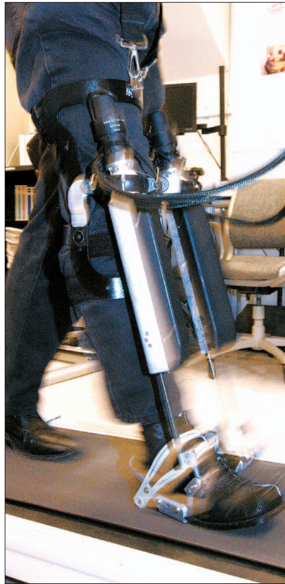
The Anklebot helps improve movement in paralyzed ankles. (photo by L. Barry Hetherington)
