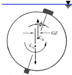
Figure 1: Righting arm (GZ) for a submerged spherical vehicle.
