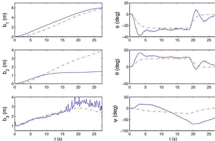
Figure 2: *Experimental (solid) and theoretical (dashed) evolutions of the AUV for the  $(STPP)_2$  strategy targeting  $\eta_T = (6, 4, 1, 0, 0, 0)$ .*
