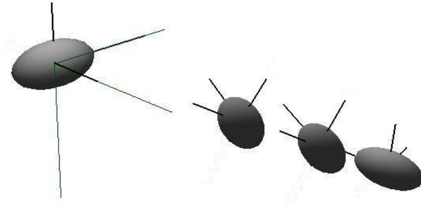
Figure 3: *Decoupling vector field trajectory using only the V thrusters, beginning at the origin and ending at  $\eta_f = (4, 3, 2, 0, 0, -90^\circ)$ .*
