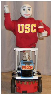
Fig. 1. Bandit, a socially assistive humanoid robot, shown mounted on a Pioneer mobile base.
