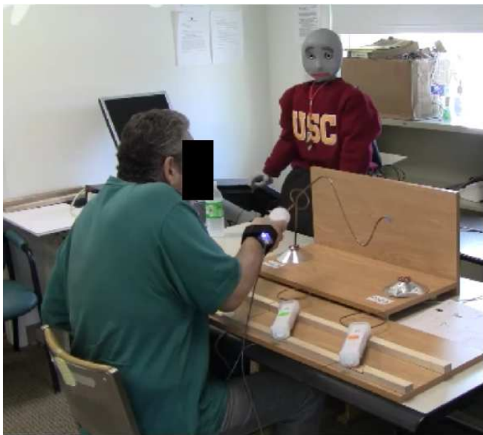
Fig. 3. A participant practicing the wire puzzle task while being guided by a socially assistive humanoid robot.
