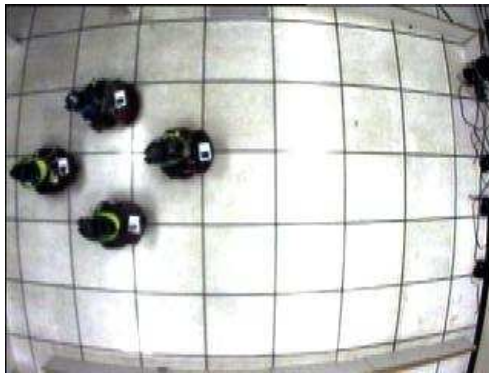
Fig. 11: An Overhead View of 4 Mobile Robots Traveling in a Diamond Formation. [10]
