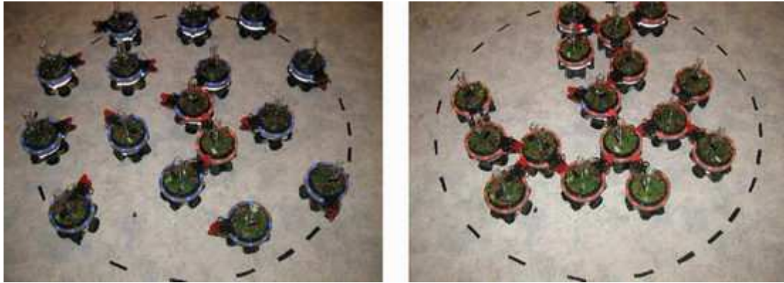
Fig. 10: Independent “Swarm-Bots” (Indicated by Blue Lights; Left) Connect with Others (Indicated by Red Lights; Right).
